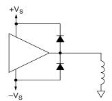
FIGURE 1. PROTECTION, INDUCTIVE LOAD
